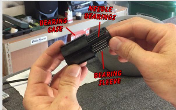
SET THE WHEEL BEARING END CAPS, AND BEACH WHEEL ASIDE. TAKE THE WHEEL BEARING CASE AND REMOVE THE BEARING SLEEVE FROM THE BEARING CASE AS SHOWN ABOVE. TRY NOT TO POP OUT THE NEEDLE BEARINGS IN THIS PROCESS.
