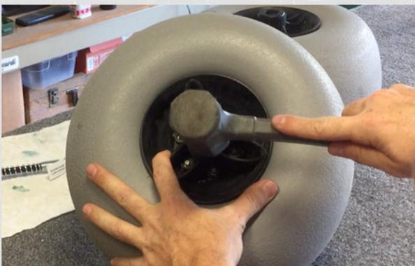
**SLIDE THE BEARING CASE BACK INTO THE WHEEL HUB WITH THE BEARING SLEEVE FACING OUT AS SHOWN ABOVE. TAKE THE BEARING CAPS AND LINE THEM UP WITH THE GROOVES OVER THE BEARING CASE AND WHEEL HUB. WITH A RUBBER Mallet GENTLY TAP TO SNAP THE BEARING CAPS BACK INTO PLACE. REPEAT THESE STEPS FOR BOTH SIDES OF EACH WHEEL.**
