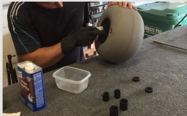
FILL YOUR CONTAINER WITH JUST ENOUGH CLEANING NAPHTHA IN A WELL VENTILATED AREA TO COVER THE PARTS. USING A PROTECTIVE GLOVE PLACE THE WHEEL BEARING CASE AND BEARING SLEEVE CONTAINING THE BEARING INTO THE NAPHTHA. GENTLY ROLL THE PARTS AROUND AND THEN CAREFULLY WIPE ANY DIRT AWAY USING A RAG AND SET THEM ASIDE. DAB A LITTLE NAPHTHA ON THE RAG AND WIPE OUT ANY DIRT INSIDE THE WHEEL HUB.
