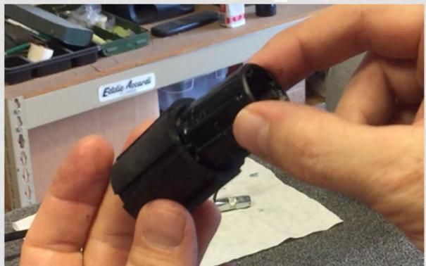
**DAB SOME MULTI PURPOSE MARINE GRADE GREASE ON YOUR FINGER AND EVENLY SPREAD IT AROUND THE OUTSIDE OF THE BEARINGS AND BEARING SLEEVE. USE JUST ENOUGH FOR A LIGHT COATING, DO NOT OVERLY USE. THEN SLIDE THE BEARING SLEEVE BACK INTO THE BEARING CASE.**
